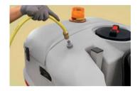
The solution hose connection with level floating ensures easy filling into the solution tank (optional)
