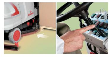
The scrubbing head assembly has two contra-rotating brushes which can swing-out laterally for easy scrubbing along walls and shelving. When impacted laterally, the brush head automatically retracts without any additional command. (it is shock absorbent). Thanks to an extremely user-friendly joystick, the scrubbing
