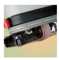
The powerful drive wheel ensures total safety. Ultra 85/100 has anti-slide wheels, speed reduction around bends, traction with control in A.C. and a watertight carbon brush-less motor all as standard features
