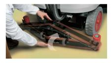
Ultra 85/100 B - Thanks to a system developed by Comac, the squeegee can be rotated by the operator till the horizontal position. This ensures a perfect cleaning of the squeegee rubbers and an excellent constant drying
