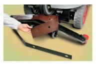
Removing the squeegee rubbers is extremely simple. Just open the hinged clamp with a hammer to easily pull out the rubber
