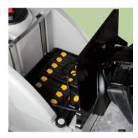
36 Volt electrical system. The large opening of the battery compartment ensures excellent accessibility and easy accommodation of the battery pack
