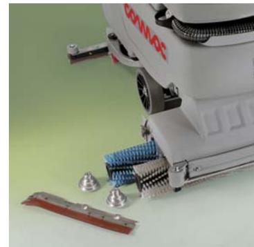
The scrubbing-sweeping head, with easily removable contra-rotating roller brushes is 50 cm wide. Solid dirt is collected and conveyed into the special removable hopper on the back
