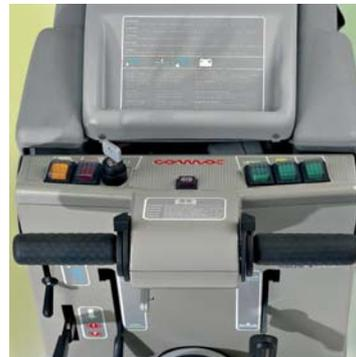
The gear-shift control is ergonomically fitted on the handle and, through a thoroughly tested electronic control, it operates the brush and the traction motor ensuring smooth operation (both in forward and reverse gear). The BT and BST versions have a parking brake pilot lamp as standard equipment
