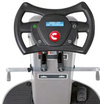
Ergonomic steering wheel with controls and display to make driving intuitive and safer, because the operator isn't distracted and the scrubbing functions are activated without ever leaving the driving wheel
